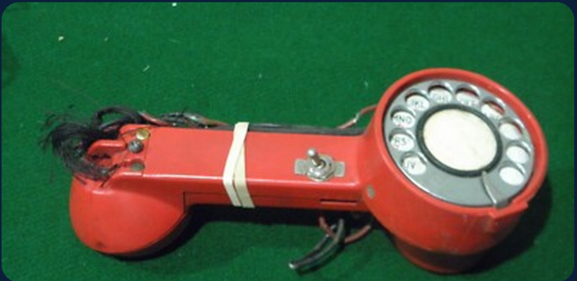
Rotary-dial lineman's test set
